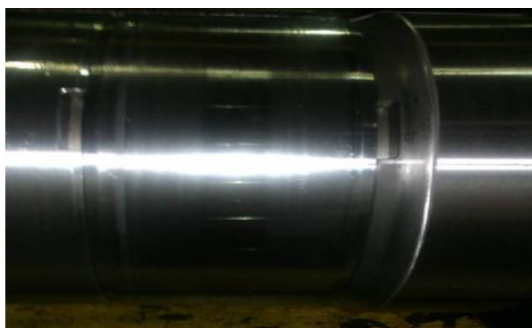
Fig: 2 Defects in work roll bearing inner races
